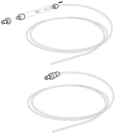
Figure 2-2. Tubing with pressure fitting assembly attached.
