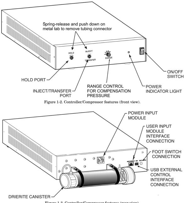
Figure 1-3. Controller/Compressor features (rear view).
